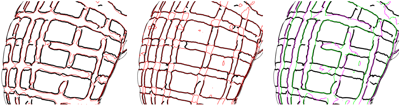
Figure 5: Demarcating curves in black, curves of zero-mean curvature (left) in red, parabolic lines (middle) in red, suggestive contours (right) in green, and suggestive highlights (right) in magenta, on the Armadillo's thigh. The thresholds are all set to zero in order to compare the curves as they are defined. The demarcating curves are closely aligned with the rectangular 3D texture, in contrast to the other curves.
