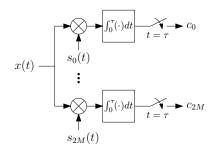
Fig. 4: Linear multichannel sampling.
