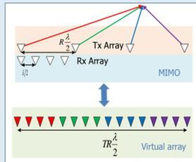
MIMO transmits orthogonal waveforms and processes linear combination of echoes received due to each waveform
