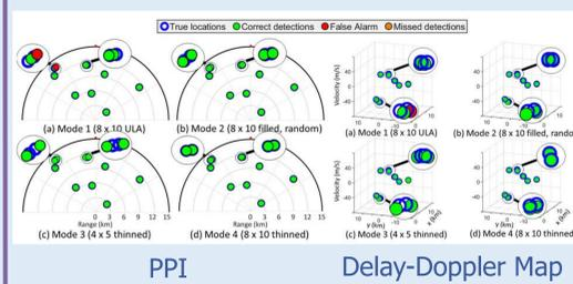
10 Targets | Min. angular spacing: 0.02 | SNR = -15 dB
