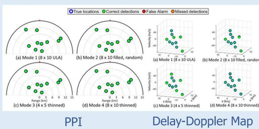
10 Targets | Min. angular spacing: 0.025 | SNR = -15 dB
