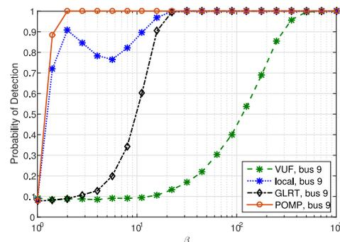
Fig. 7. Loading imbalances for IEEE 118-bus system: Probability of detection for single-phase magnitude imbalance at buses 3, 9, 33, 39, 51, 57, 75, 93, 96, 98 with  $N = 10$  and  $\text{SNR} = 10$  db. The local method is based on the single PMU located at bus 9 and the VUF and GLRT on bus 9 voltage three-phase measurements.
