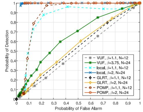
Fig. 4. Loading imbalances for IEEE 14-bus system: The ROC curves of VUF, GLRT, local MDL, and POMP for detection of single-phase magnitude imbalance at bus 9, with 1)  $\beta = 3.75$  and  $N = 24$  (solid line); and 2)  $\beta = 1.1$  and  $N = 12$  (dashed line). The local method is based on the single PMU located at bus 7.
