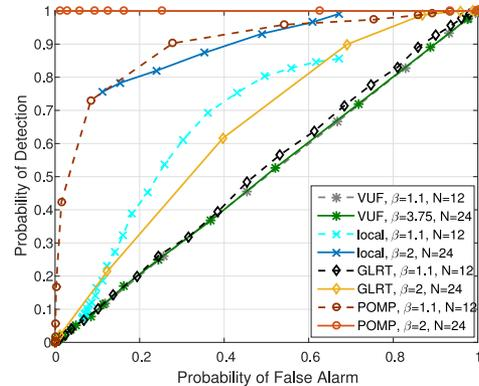
Fig. 6. Loading imbalances for IEEE 118-bus system: The ROC curves of VUF, GLRT, local MDL, and POMP methods for detection of single-phase magnitude imbalance at bus 9, with 1)  $\beta = 3.75$  and  $N = 24$  (circle); and 2)  $\beta = 1.1$  and  $N = 12$  (diamond). The local method is based on the single PMU located at bus 9.
