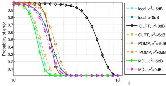
Fig. 3. Two-port  $\pi$ -model: Probability of error for two-port  $\pi$ -model with  $\sigma^2 = -5, 0$  dB,  $N = 48$ , and single-phase voltage magnitude imbalance at bus 2.
