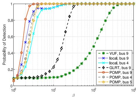
Fig. 5. Loading imbalances for IEEE 14-bus system: Probability of detection for  $N = 10$  and  $\text{SNR} = 10$  db, single-phase magnitude imbalance at buses 4, 5 and 9, and PMUs at buses 2, 6, 7, 9. The local method is based on the single PMU located at bus 7 and the VUF and GLRT on bus 9 voltage three-phase measurements.
