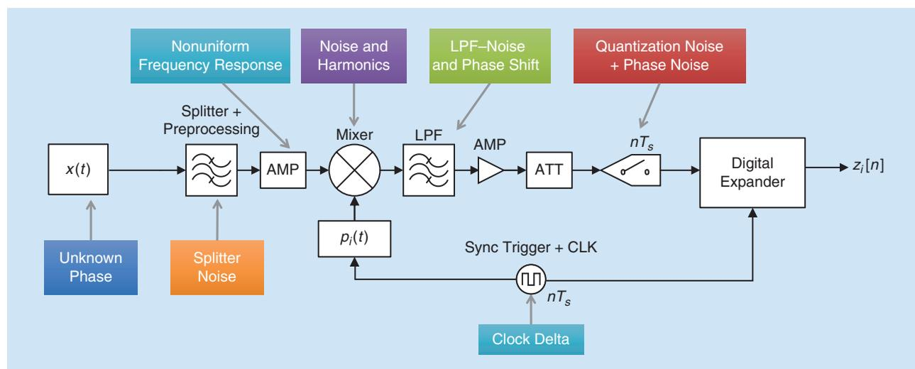
**FIGURE 13.** The hardware RF chain detailed schematics, including the amplifiers, attenuators, filters, mixers, samplers, and synchronization signals required for precise and accurate operation. The distortions induced by each component are indicated as well. Freq.: frequency; ATT: attenuator; CLK: clock.
