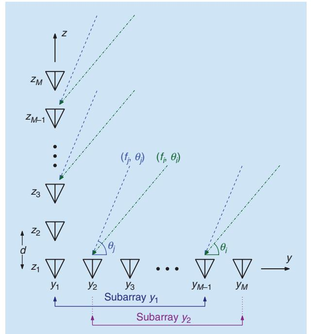
**FIGURE 25.** The GaSCADE system: an L-shaped array with  $M$  sensors along the  $y$  axis and  $M$  sensors along the  $z$  axis, including a common sensor at the origin. The subarrays  $\mathbf{y}_1$  and  $\mathbf{y}_2$  (and similarly  $\mathbf{z}_1$  and  $\mathbf{z}_2$ ) are defined in the derivation of the 2-D-ESPRIT algorithm.
