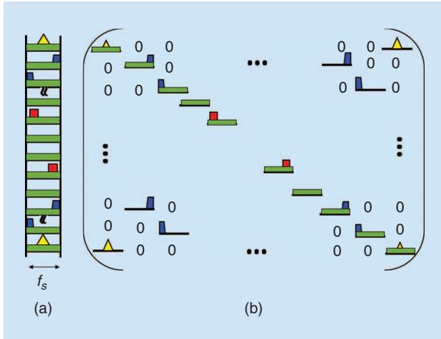
**FIGURE 18.** (a) The spectrum slices vector  $x(\tilde{f})$  and (b) correlated slices of  $x(\tilde{f})$  in the matrix  $\mathbf{R}_x^a(\tilde{f})$ .
