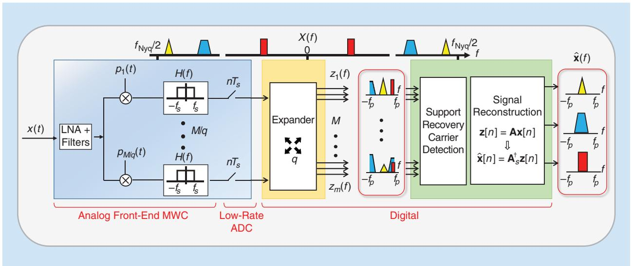
**FIGURE 9.** A schematic implementation of the MWC analog sampling front end and digital signal recovery from low-rate samples. LNA: low-noise amplifier.
