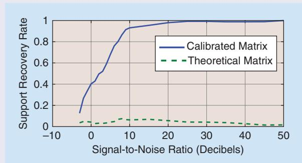
**FIGURE S3.** The hardware reconstruction success rate of the calibrated matrix versus the theoretical matrix.
