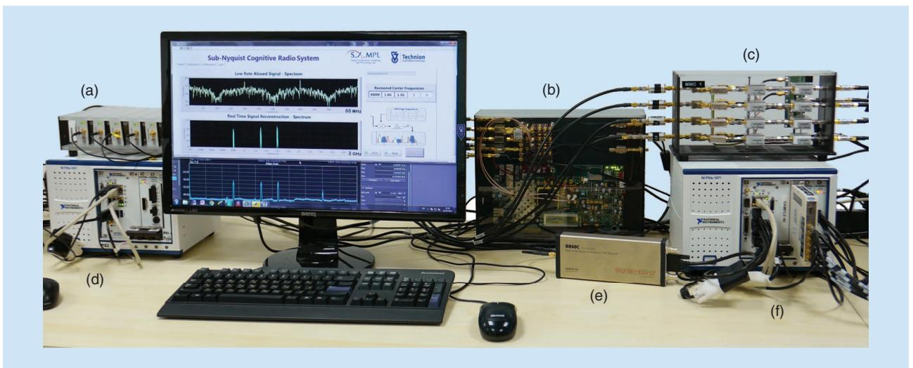
**FIGURE 12.** The MWC CR system prototype: (a) vector signal generators, (b) an FPGA mixing sequences generator, (c) an MWC analog front-end board, (d) an RF combiner, (e) a spectrum analyzer, and (f) an ADC and digital signal processor digital signal processor.
