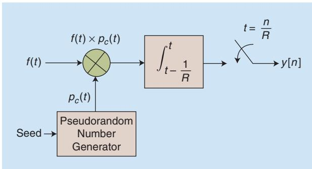
**FIGURE 3.** A block diagram for the random demodulator, including a random number generator, a mixer, an accumulator, and a sampler [23].
