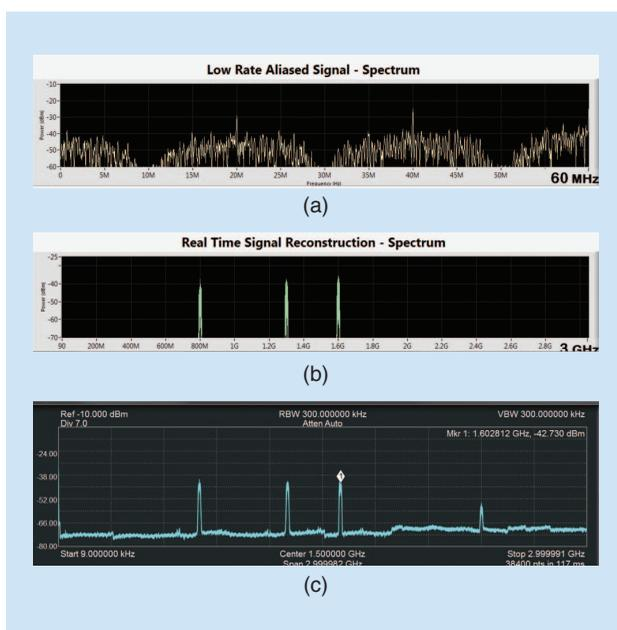
**FIGURE 14.** A screenshot from the MWC recovery software: (a) low-rate samples acquired from one MWC channel at rate 120 MHz; (b) digital reconstruction of the entire spectrum, performed from sub-Nyquist samples; and (c) true input signal  $x(t)$  showed using a fast spectrum analyzer.
