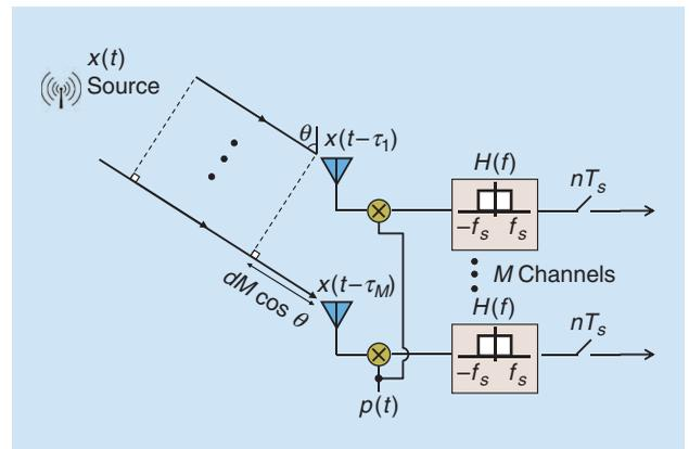
**FIGURE 10.** A uniform linear array configuration with  $M$  sensors, with the distance  $d$  between two adjacent sensors. Each sensor includes an analog front end composed of a mixer with the same periodic function  $p(t)$ , an LPF, and a sampler at the rate  $f_s$ .
