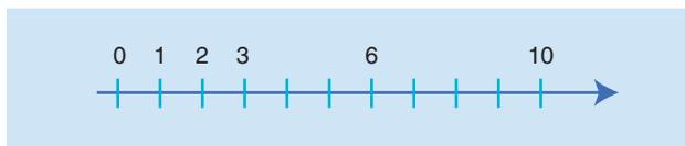
FIGURE 17. A minimal sparse ruler of order  $M = 6$  and length  $N = 10$ .
