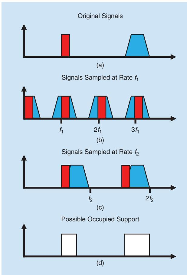
**FIGURE 4.** The action of the SMRS on a multiband signal. (a) The input signal with  $K = 2$  bands, (b) signals sampled at rate  $F_1$  in channel 1, (c) signals sampled at rate  $F_2$  in channel 2, and (d) possible support that is the intersection of the supports in channels 1 and 2 [24].
