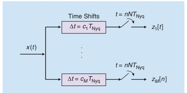
FIGURE 6. A schematic implementation of multicoset sampling. The input signal  $x(t)$  is inserted into the multicoset sampler, which splits the signal into  $M$  branches and delays each one by a fixed coefficient  $c_i T_{\text{Nyq}}$ . Every branch is then sampled at the low rate  $1/(NT_{\text{Nyq}})$  and then digitally processed to perform spectrum sensing and signal reconstruction.
