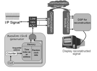
Fig. 2. Diagram of the random sampling ADC. A pseudorandom clock generated by an FPGA drives a low-rate standard ADC to sample the input signal at predetermined pseudorandom times. The samples obtained are then fed into a CS recovery algorithm or a sketching algorithm for Fourier sparse signals to estimate the frequencies and amplitudes of the tones present in the signal (taken from [81]).
