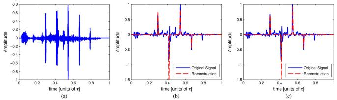
Fig. 17. Applying the SoS sampling scheme with  $b_k = 1$  on real ultrasound imaging data. Results are shown versus original signal which uses 4160 samples. (a) Recorded ultrasound imaging signal. The data was acquired by GE healthcare's Vivid-i ultrasound imaging system. Reconstructed signal (b) using N = 17 samples and (c) using N = 33 samples (taken from [163]).
