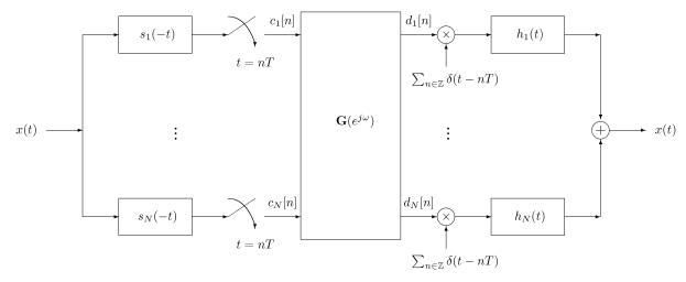
Fig. 11. Sampling and reconstruction in shift-invariant spaces. A compressive signal acquisition scheme can be obtained by reducing the number of sampling filters from N to p < N and replacing the filter bank  $G(e^{j\omega})$  with a CTF block with real-time recovery (taken from [18]).
