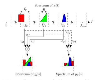
Fig. 12. Spectrum slices of x(t) are overlayed in the spectrum of the output sequences  $y_i[n]$ . In the example, channels *i* and *i'* realize different linear combinations of the spectrum slices centered around  $lf_p$ ,  $\bar{l}f_p$ ,  $\bar{l}f_p$ . For simplicity, the aliasing of the negative frequencies is not drawn (taken from [9]).
