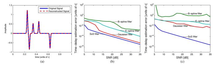
Fig. 15. Performance comparison of finite pulse stream recovery using Gaussian [6], B-spline, E-spline [7], and SoS sampling kernels. (a) Reconstructed signal using SoS filters versus original one. The reconstruction is exact to numerical precision. (b) L = 3 Dirac pulses are present, (c) L = 5 pulses (taken from [163]).
