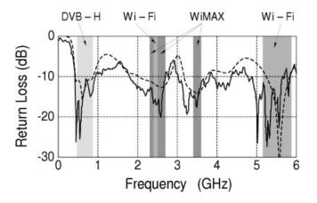
**Figure 2** Simulated and measured input return loss of the proposed multiband antenna when it is free-standing: simulated (dashed line) and measured (solid line)
