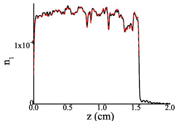
Fig. 4. (Color online) Amplitude of the reconstructed grating performed from the two grating sides. The solid curve corresponds to the data shown in Figs. 1 and 2, whereas the dashed curve corresponds to the reconstruction from the other side of the grating. The figure shows an excellent agreement between the two reconstructions. The maximum difference between the two reconstructed amplitude profiles is equal to 4% of the maximum grating amplitude.
