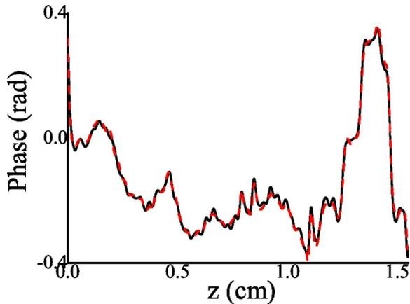
Fig. 5. (Color online) Phase of the reconstructed grating performed from the two grating sides. The maximum difference between the two reconstructed phase profiles is 0.03 rad. Curve definitions as in Fig. 4.
