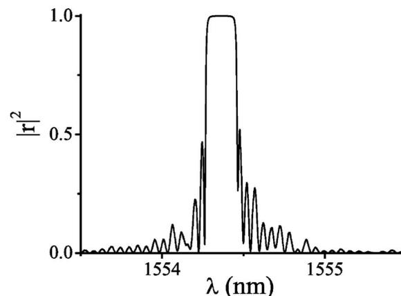
Fig. 3. Intensity of the measured complex reflection spectrum after performing spectrum regularization.
