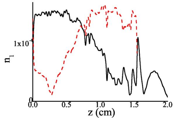
Fig. 7. (Color online) Grating amplitude, reconstructed from both grating sides when the reflection spectrum is regularized, but the DLP algorithm is used instead of the ILP algorithm. The figure shows that the grating cannot be reconstructed using the DLP algorithm. Thus, it is essential that the ILP algorithm be used. Curve definitions as in Fig. 4.
