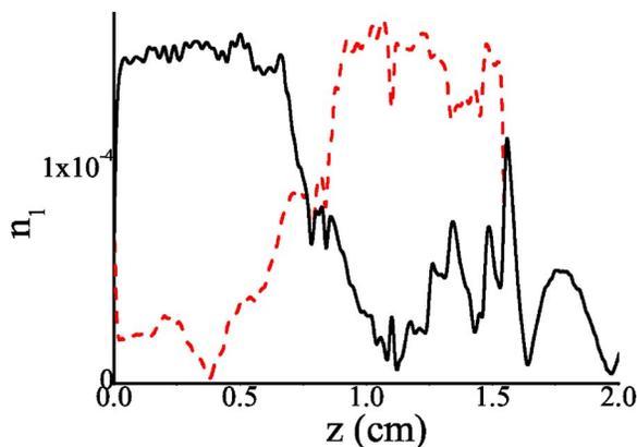
Fig. 6. (Color online) Grating amplitude, reconstructed from both grating sides when the reflection spectrum is not regularized and the ILP algorithm is used. The figure shows that the grating cannot be reconstructed without regularizing its reflection spectrum. Curve definitions as in Fig. 4.
