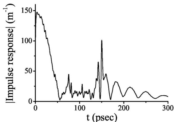
Fig. 2. Amplitude of the grating impulse response. The discontinuity at approximately  $t=150$  ps is caused by a reflection from the grating end.
