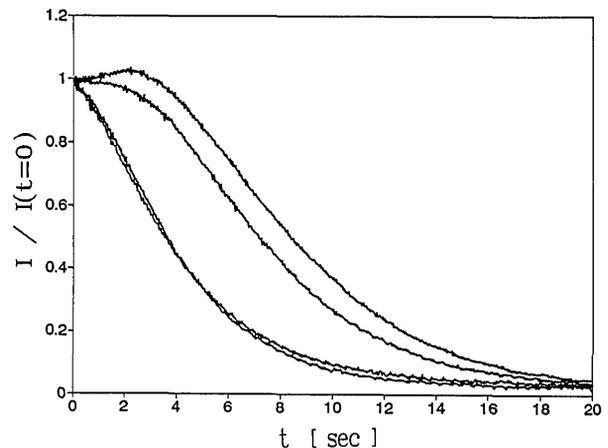
Fig. 5. Experimental results of the (normalized) signal output decay when the input signal is turned off, for various signal-to-pump ratios  $I_4/I_1$ :  $2 \times 10^{-5}$ ,  $4 \times 10^{-5}$ ,  $1.5 \times 10^{-4}$ , and  $3 \times 10^{-4}$ . Curves with slower decays correspond to higher ratios.
