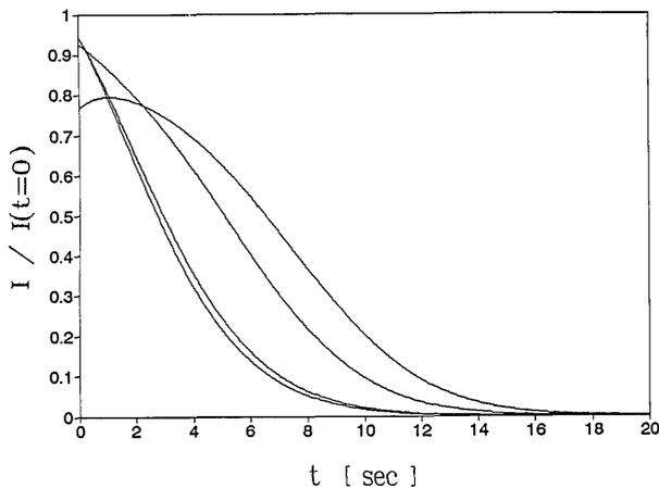
Fig. 7. Theoretical results of the (normalized) signal output decay when the input signal is turned off for various signal-to-pump ratios  $I_4/I_1$ :  $2.5 \times 10^{-5}$ ,  $2.8 \times 10^{-4}$ ,  $1/100$ , and  $1/9$ . The coupling constant used in these curves is the estimated  $\gamma l = 3.6$  from the small-signal experimental curves of buildup and erasure (Figs. 2 and 3). Curves with slower decays correspond to higher ratios.
