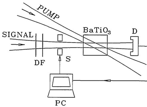
Fig. 1. Schematic of the experimental setup. DF, neutral-density filter; S, shutter; PC, personal computer; D, detector. The pump and the signal beams are denoted as 1 and 4, respectively, in the text.
