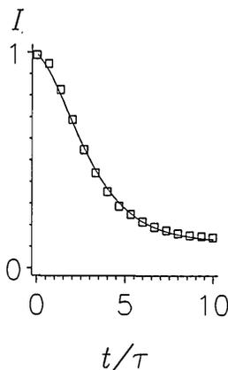
Fig. 3. Experimental data and a theoretical fit of the (normalized) signal output decay for the small-signal regime with a signal-to-pump ratio of  $I_4/I_1 = 9.7 \times 10^{-6}$ . As for Fig. 2, the signal includes the fanning and does not decay to a zero value.
