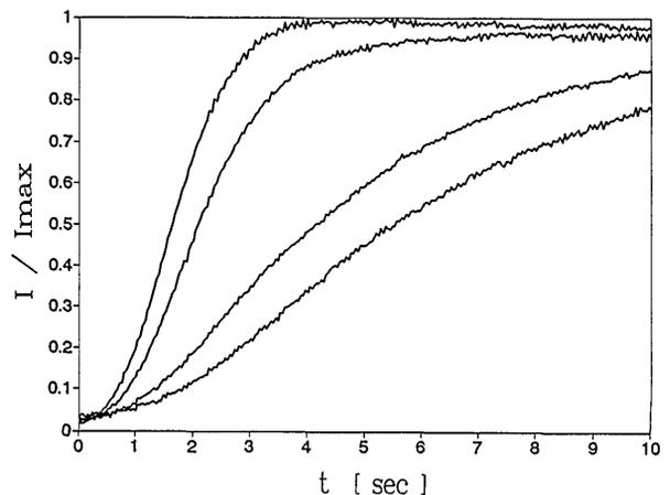
Fig. 4. Experimental results of the (normalized) signal output buildup for various signal-to-pump ratios  $I_4/I_1$ :  $2 \times 10^{-5}$ ,  $4 \times 10^{-5}$ ,  $1.5 \times 10^{-4}$ , and  $3 \times 10^{-4}$ . Curves with quicker buildups correspond to higher ratios.
