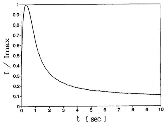
Fig. 8. Experimental results showing the long-term buildup of the signal, taken for high signal-to-pump ratios of  $1/10$ . (The intensity  $I$  is in arbitrary units). Here we see the strong depletion of the signal beam caused by the fanning (amplified noise) buildup, which has a slower response.
