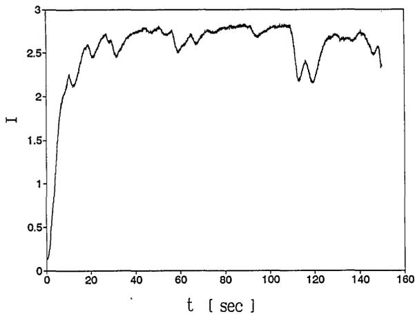
Fig. 9. Experimental data for the signal output buildup for strong input beams, showing the fluctuations that are due to thermal changes in the crystal. Here the pump power was 50 mW, compared with 10 mW in all other experiments.
