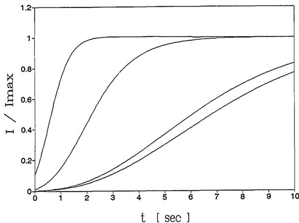
Fig. 6. Theoretical results of the (normalized) signal output buildup for various signal-to-pump ratios  $I_4/I_1$ :  $2.5 \times 10^{-5}$ ,  $2.8 \times 10^{-4}$ ,  $1/100$ , and  $1/9$ . The coupling constant used in these curves is the estimated  $\gamma l = 3.6$  from the small-signal experimental curves of buildup and erasure (Figs. 2 and 3). Curves with quicker buildups correspond to higher ratios.
