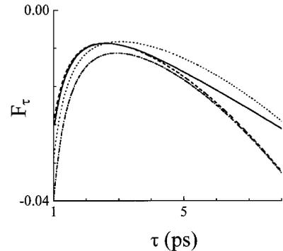
Fig. 1. Cavity loss depending on the pulse duration,  $F_\tau$ , versus the FWHM of pulse duration,  $\tau$ , obtained from the numerical model (solid curve), from soliton perturbation theory (dashed-dotted curve), and from Eq. (3) for a hyperbolic-secant pulse (dashed curve) and a Gaussian pulse (dotted curve).
