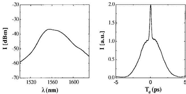
Fig. 1. Optical spectrum and the corresponding background free autocorrelation trace for a noiselike mode with short pulses.
