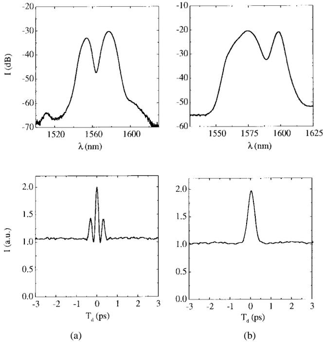
Fig. 3. Optical spectrum and the corresponding background free autocorrelation trace in a two-color operation mode (a) for the coherent mode and (b) for the incoherent mode. For both modes a dispersion shifted fiber was used.
