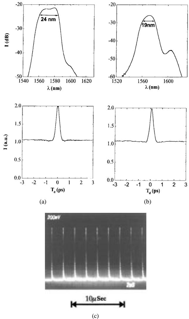
Fig. 2. Optical spectrum, the corresponding background free autocorrelation trace and the pulse train: (a) with 450-m dispersion shifted fiber added to the cavity and (b) with 450 m of a dispersive fiber (Corning SMF28) added.
