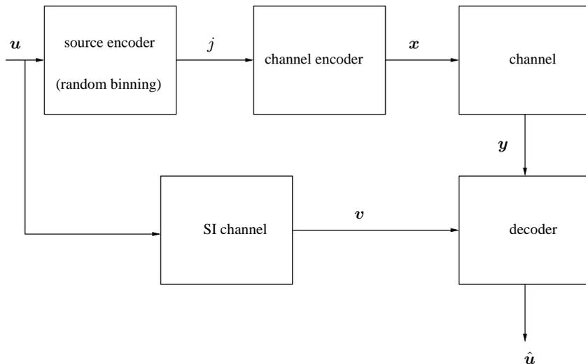
Figure 1: Slepian–Wolf source coding, followed by channel coding. The source  $\mathbf{u}$  is source–channel encoded, whereas the correlated SI  $\mathbf{v}$  (described as being generated by a DMC fed by  $\mathbf{u}$ ) is available at the decoder.
