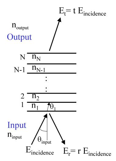
The idea is that the propagation of the electromagnetic field through a structure is described by a characteristic matrix (M). M relates the field (E and H) at the input plane to that at the output plane (input=M\*output). If a structure is complex (like multi-layer system) the equation becomes: input= $M_1*M_2*...M_{N-1}*M_N*$  output, where  $M_N$  describes the layer that is closest to the output plane or in other words  $M=M_1*M_2*...M_{N-1}*M_N$ .
