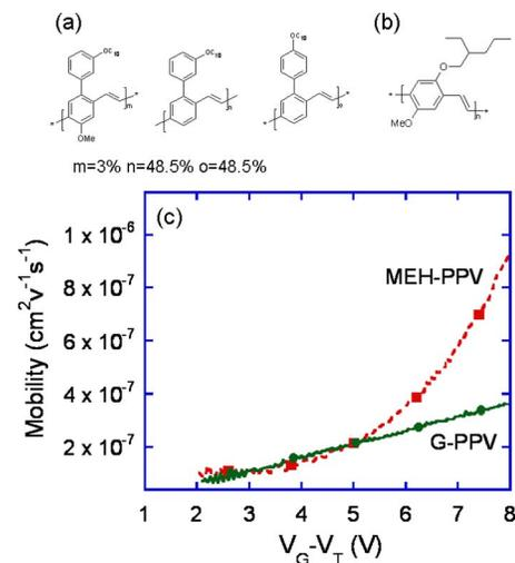
FIG. 2. (Color online) (a) Chemical structure of green PPV. (b) Chemical structure of MEH-PPV. (c) Hole field effect mobility extracted from the transfer characteristics of bottom contact FETs (Ref. 15).
