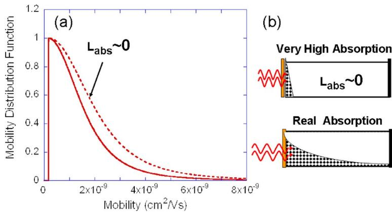
FIG. 1. (Color online) (a) Electron mobility distribution function extracted for MEH-PPV based device. The dashed line is derived using Eq. (1) and does not account for the finite absorption depth of the polymer. The full line is derived using Eq. (3) and represents the true MDF. (b) Illustration of a device with infinitely high absorption coefficient (top) and a more realistic case (bottom).
