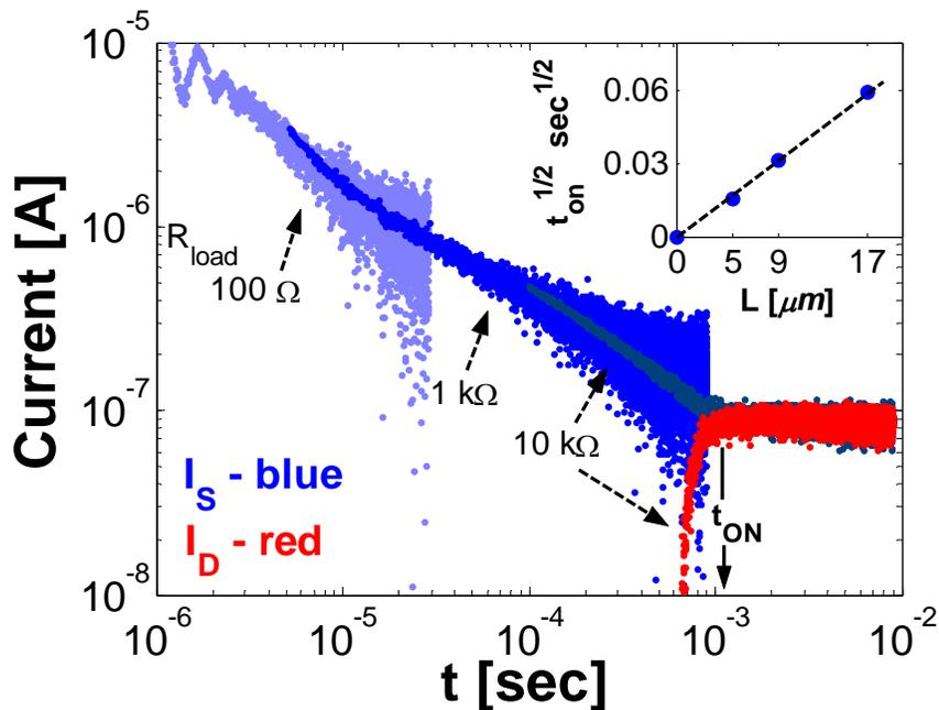
**Figure 3:** Measured source (blue) and drain (red) currents of PFET after switching the gate voltage from 0 V to -8 V where the drain voltage was kept at constant bias ( $V_{DS}=-8$  V). The switching time ( $t_{on}$ ) is the time that drain current reaches its DC value, the channel charging is completed and the source and the drain currents are equal. The switch on time is scaled with the squared channel length (see insert).
