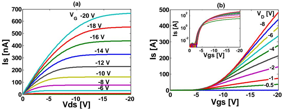
**Figure 2:** Conductance (a) and transconductance (b) characteristics of 17.5 [ $\mu\text{m}$ ] channel MEH-PPV CI $\pi$ -FET. (The saturation mobility  $\mu_{\text{sat}} = 2 \cdot 10^{-4}$  [ $\text{cm}^2 / \text{V sec}$ ])
