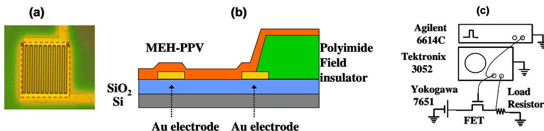
**Figure 1:** Top view (a) of MEH-PPV PFET with periphery current reduction by polyImide field insulator. The active area, marked by a dashed line in (a), is surrounded by field insulator, as plotted in the schematic cross section near the active area edge (b). The time response measurement setup is given in (c).
