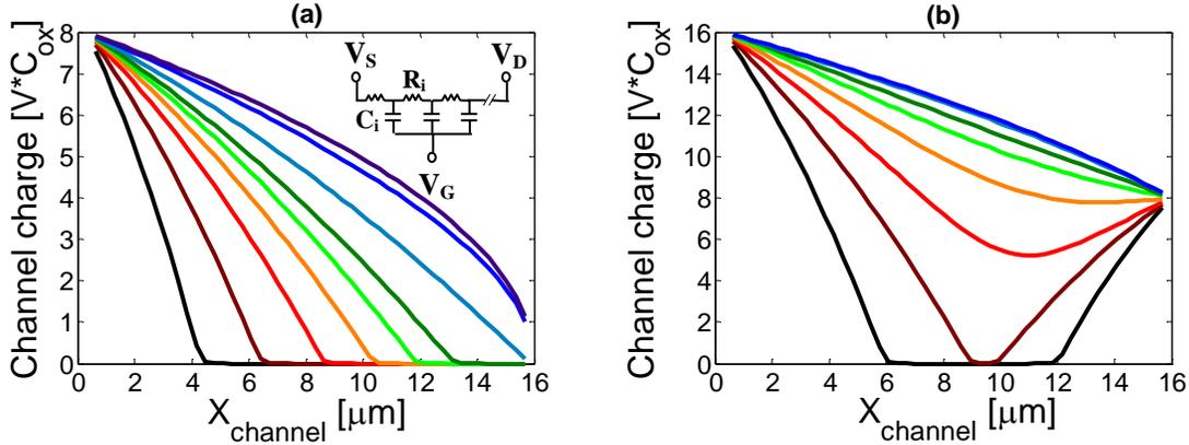
**Figure 4:** Transmission line method (TLM) Calculated surface charge in the FET channel at different elapsed times after operating gate bias for: (a) low drain voltage ( $|V_{GS} - V_T| \leq |V_{DS}|$ ,  $V_{GS} = V_{DS} = -8$  [V],  $V_T = 0$ ), and (b) high gate voltage ( $|V_{GS} - V_T| > |V_{DS}|$ ,  $V_{GS} = -16$  [V],  $V_{DS} = -8$  [V],  $V_T = 0$ ). The colors at both graphs present the same elapsed time after gate bias switching.
