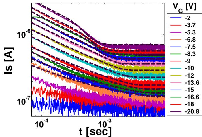
**Figure 5:** Experimental and transmission line simulation results (colored and dashed lines, respectively) of PFET charging current for different gate voltages ( $V_D = -8$  [V]). All of the simulation are with the same parameters:  $V_T = -3.6$  [V],  $\mu = 1.4 \cdot 10^{-4}$  [ $\text{cm}^2 / \text{V sec}$ ], and  $I_{noise} = 9 \cdot 10^{-8}$  [A].
