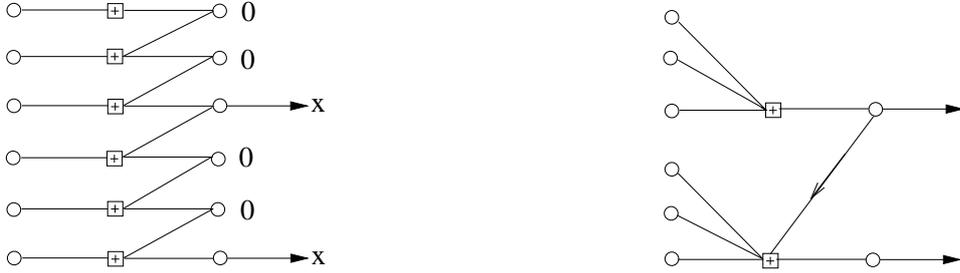
Figure 2.4: Accumulate code with puncturing period  $p = 3$  and an equivalent version of an  $\text{SPC}(p)$  code followed by an accumulate code.
