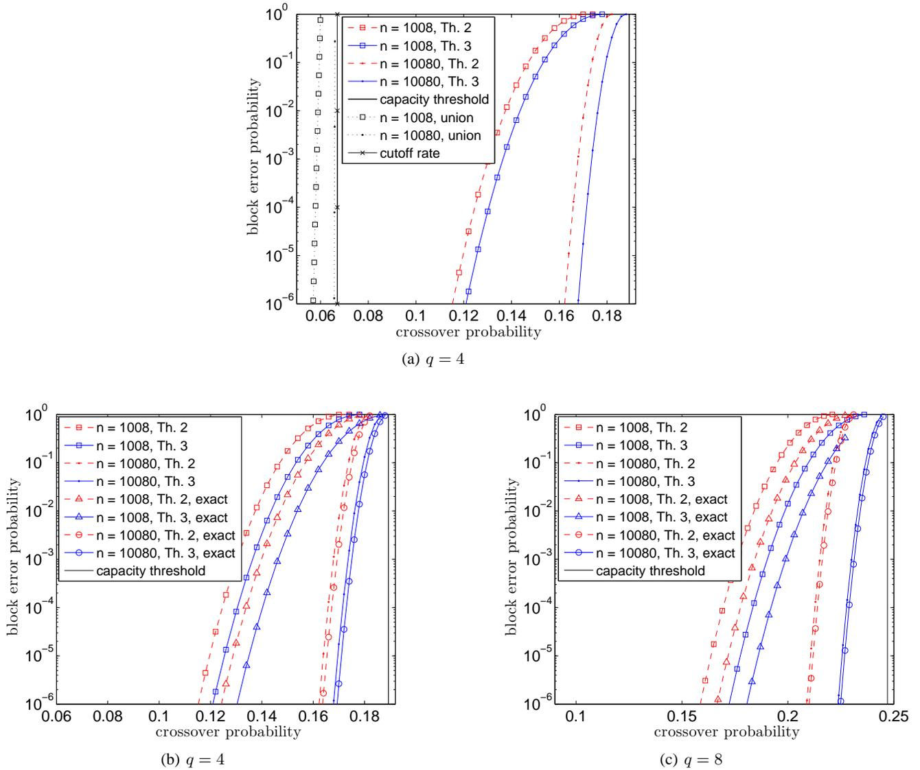
Fig. 1: Upper bounds on the block error probability of the Gallager (8, 16) regular and non-binary LDPC code ensembles with quaternary and octal input alphabets. The transmission takes place over a  $q$ -ary symmetric channel where  $q = 4$  in plots (a) & (b) and  $q = 8$  in plot (c). This figure refers to expurgated ensembles whose block lengths are 1008 and 10,080 symbols.
