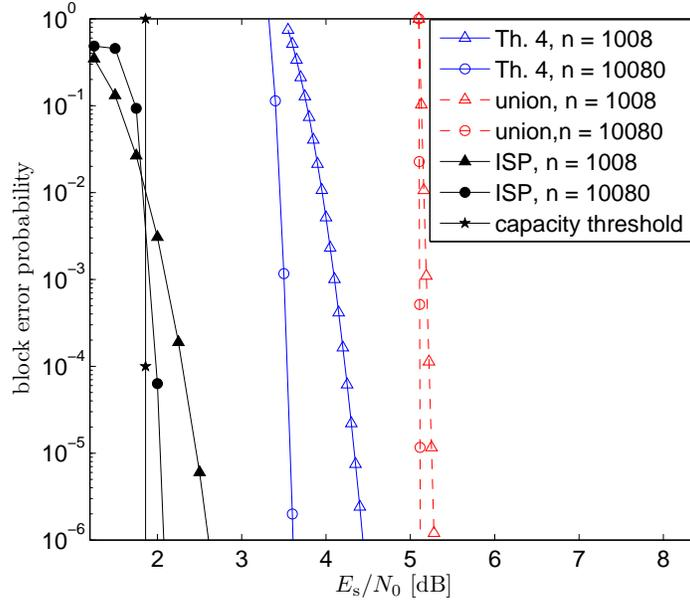
Fig. 7: A comparison between the DS2 and union upper bounds on the block error probability under ML decoding for the  $(8, 16)$ -regular LDPC ensemble of Gallager (see Example 7). The transmission takes place over fully-interleaved Rayleigh fading channel with a QPSK modulation and perfect CSI at the receiver. The ISP lower bounds on the decoding error probability are shown for block lengths of 1008 and 10080 symbols. The capacity limit for infinite block length is also presented as a reference.
