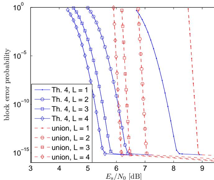
Fig. 6: Upper bounds on the block error probability under ML decoding for the (8,16)-regular LDPC ensemble of Gallager with octal alphabet and a block length of 1008 symbols. The transmission takes place over a fully-interleaved Rayleigh fading channel with 8-ary PSK modulation, perfect CSI and maximal ratio combining (MRC) at the receiver. The figure depicts the performance for MRC diversity with  $L = 1$  to  $L = 4$  antennas at the receiver.
