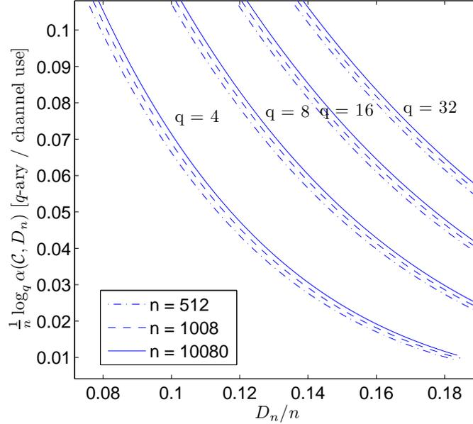
Fig. 3: The term  $\frac{1}{n} \log_q \alpha(\mathcal{C}, D_n)$  in (12) for the regular (8,16) LDPC ensemble of Gallager [22], depicted for alphabet sizes of  $q = 4, 8, 16,$  and  $32,$  and block lengths of  $n = 512, 1008,$  and  $10080$  symbols.
