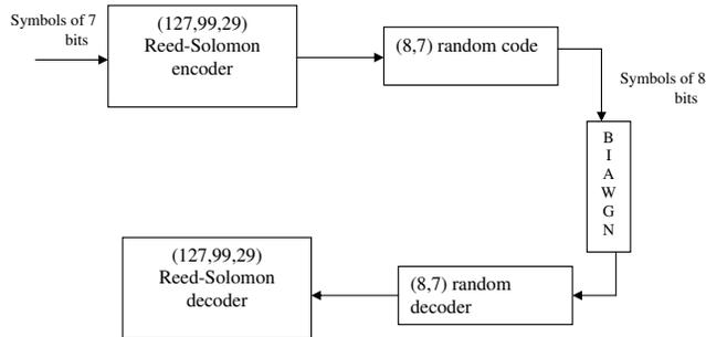
Fig. 2. A scheme for an ensemble of serially concatenated codes where the outer code is a  $(127, 99, 29)$  Reed-Solomon (RS) code, and the inner code is chosen uniformly at random from the ensemble of  $(8,7)$  binary linear block codes.
