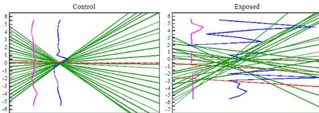
Good quality lens as demonstrated by the optical scanner. All rays passing Through the lens have similar focal length. The thick dashed line connects the points of the back vertex Distance for each ray passing through the lens. The thick solid line shows the relative intensity of each beam.
