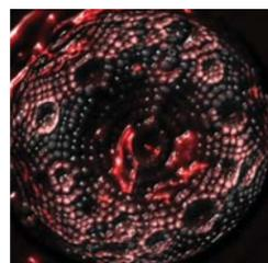
Furthermore, what  $N_2$  is present near the tip helps to stabilize the tungsten against further chemical degradation. Indeed, the resultant needle is stable up to temperatures of 900 degrees Celsius even after 24 hours of exposure to air.
