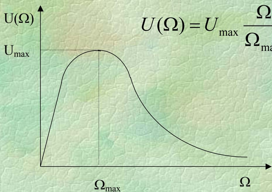
$$U(\Omega) = U_{\max} \frac{\Omega}{\Omega_{\max}} \exp\left(-\frac{\Omega - \Omega_{\max}}{\Omega_{\max}}\right)$$
