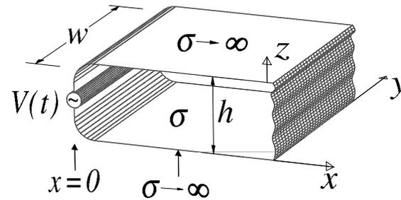
Figure 4.3: Model of a quasi-static resistor.
