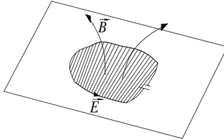
Figure 1.4: Flux through a metallic loop.
