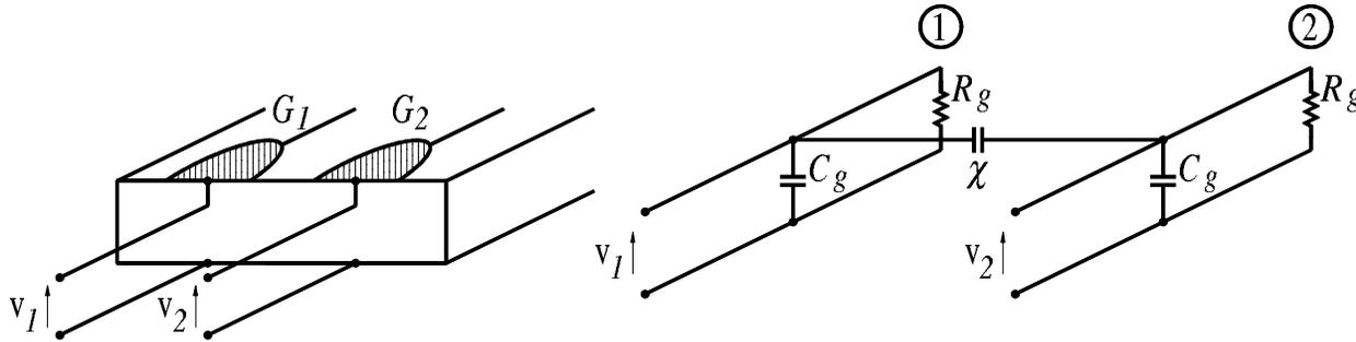
Figure 5.7: Two gates that may become coupled (left) and the equivalent circuit that describes their operation.
