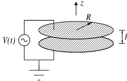
Figure 3.1: Simple model for a capacitor.
