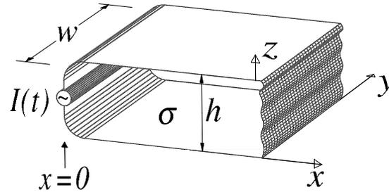
Figure 4.4: Basic setup for demonstration of a transient phenomena in a metallic medium.
