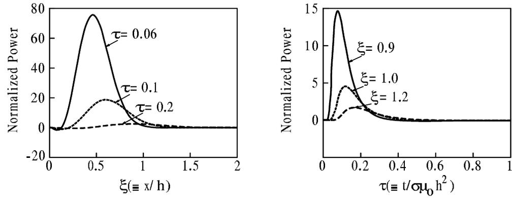
Figure 4.6: Penetration of the dimensionless power in space (left) and in time (right).
