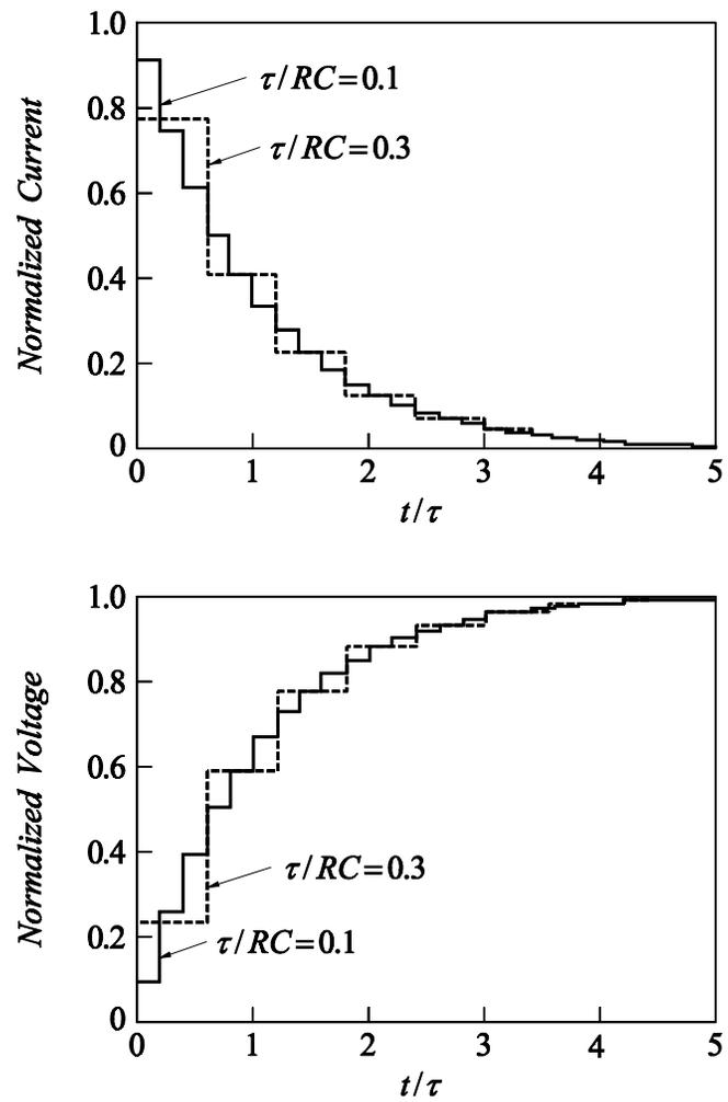
Figure 4.8: Time variation of the current and voltage at the input of the lumped capacitor.
