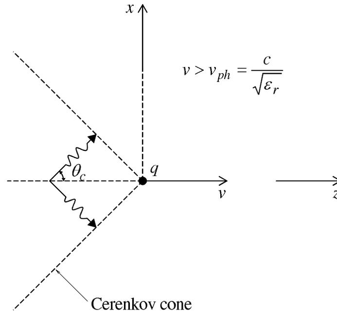
Figure 8.1: Charge that moves in a dielectric medium faster than the speed of light,  $c/\sqrt{\epsilon_r}$ , in that medium, generates Cerenkov radiation.
