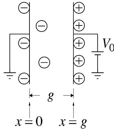
Figure 7.B.1: Vacuum diode.
