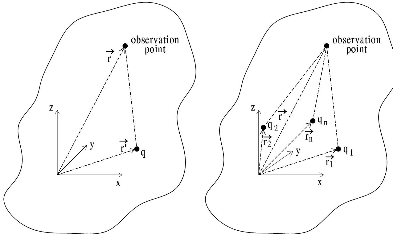
Figure 6.1: Potential generated by a point-charge and several point-charges at a given place in space.
