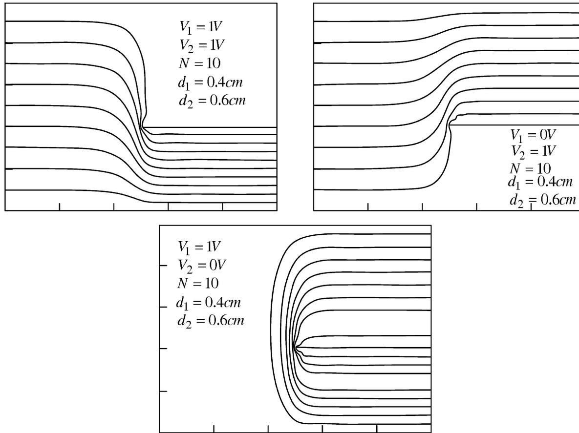
Figure 5.4: The potential contours occurring between the metallic plates.
