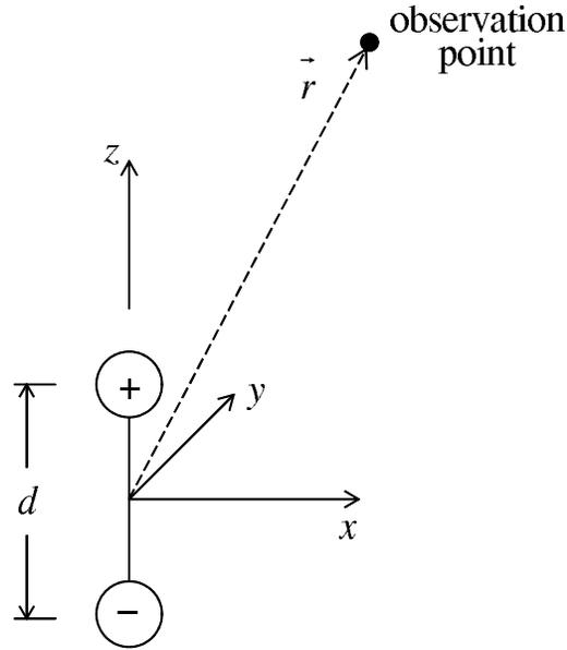
Figure 7.1: Two charges ( $\pm q$ ) separated by a distance  $d$  form a dipole moment  $p = qd$ . Since the dipole moment is a vector in this particular case  $\vec{p} = qd\vec{1}_z$ .
