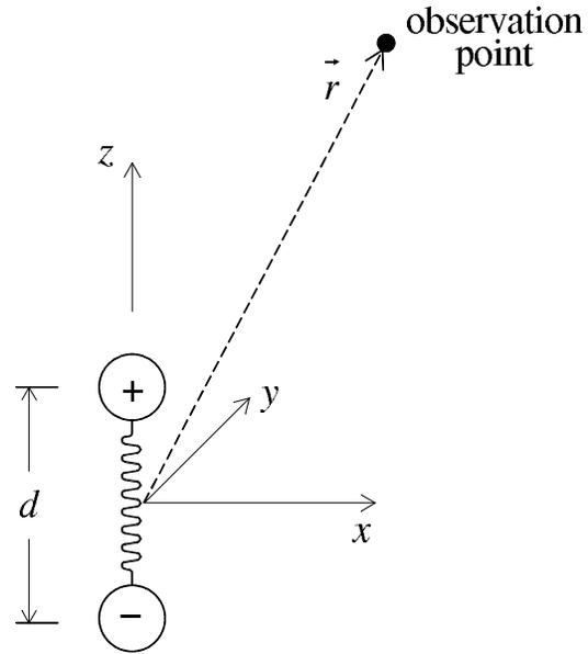
Figure 8.2: Oscillating dipole.
