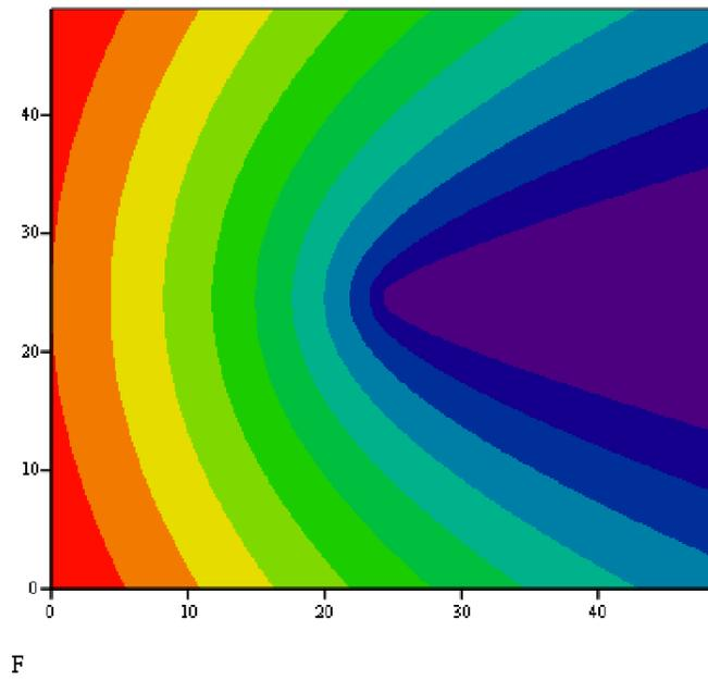
Figure 7.6: Contours of constant potentials in the vicinity of an edge of an angle  $30^\circ$ .
