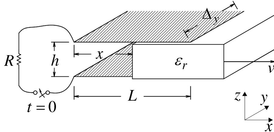
Figure 7.3: A dielectric layer moves between the two plates of a capacitor.
