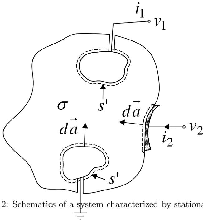
Figure 5.12: Schematics of a system characterized by stationary conductive coupling.
