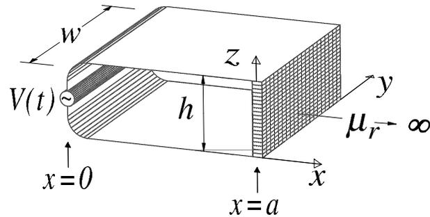
Figure 4.1: Model of a quasi-static capacitor.
