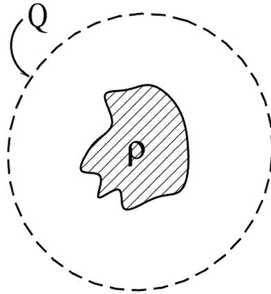
Figure 1.6: The total charge enclosed in a surface is directly linked to the electric induction.
