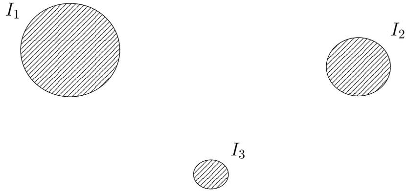
Figure 5.15: Three wires with the third providing the return path to the other two currents.
