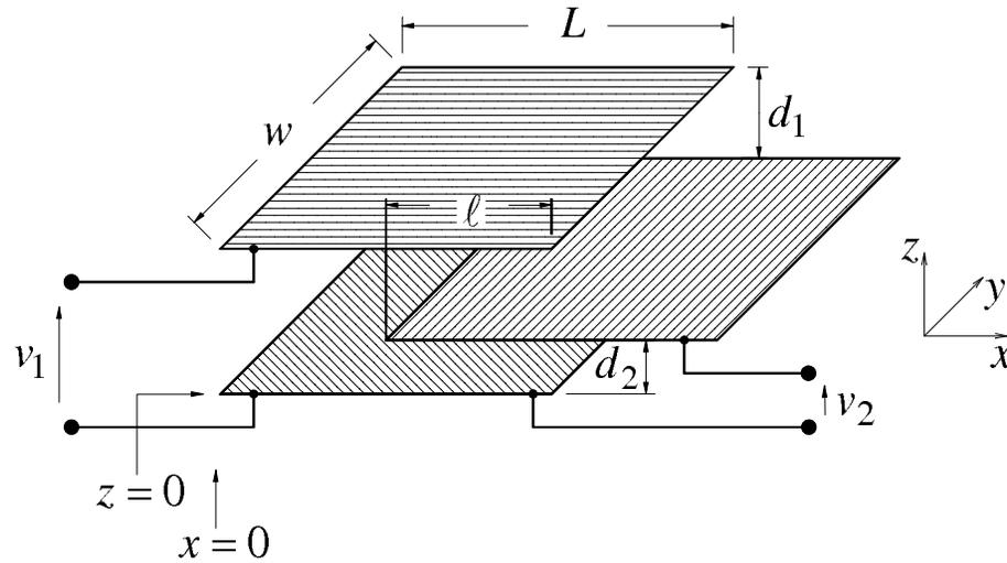
Figure 5.2: Simple electro-static coupling example.
