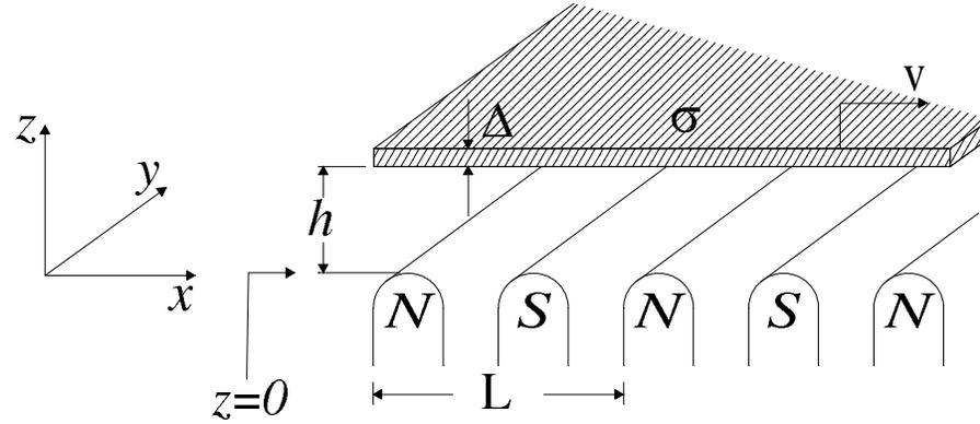
Figure 7.14: Metallic plate moving above an array of periodic magnets.
