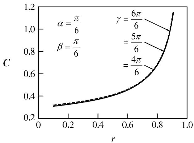
Figure 7.11: Capacitance as a function of the various parameters.
