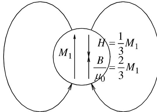
Figure 7.A.4: The magnetic field in the material is anti-parallel to the magnetization field.
