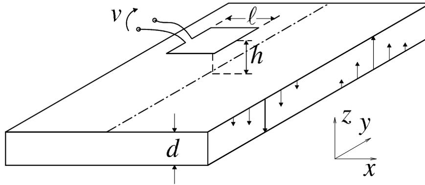
Figure 7.4: The magnetic flux imprinted in a moving tape is measured as voltage by a suspended loop.
