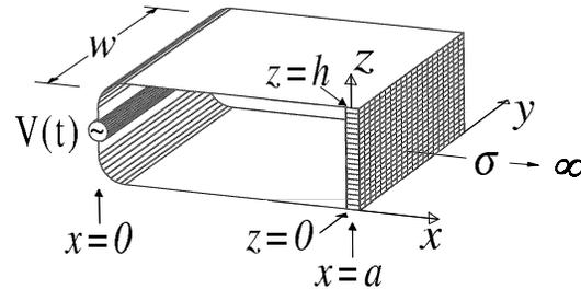
Figure 4.2: Model of a quasi-static inductor.
