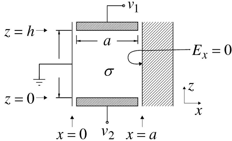
Figure 5.13: Simple model for conductive coupling.
