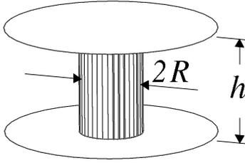
Figure 3.2: Simple model for a resistor.
