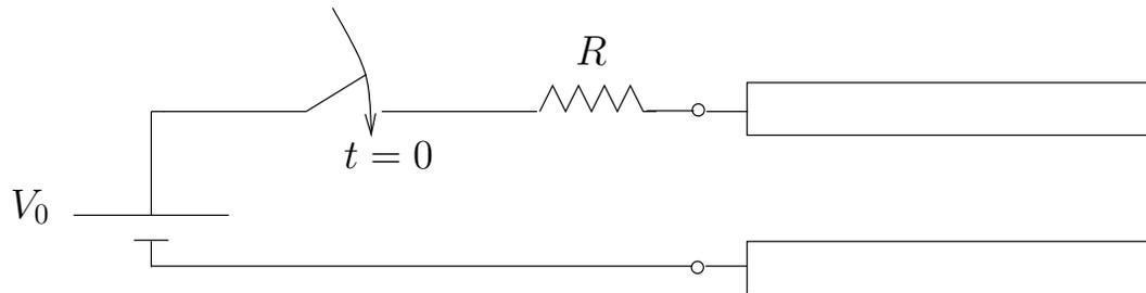
Figure 4.7: Charging of a lumped capacitor.
