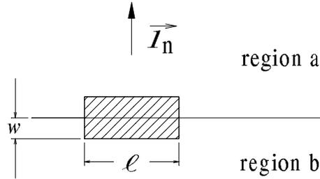
Figure 1.8: Surface charge density is linked to the discontinuity in perpendicular electric induction.
