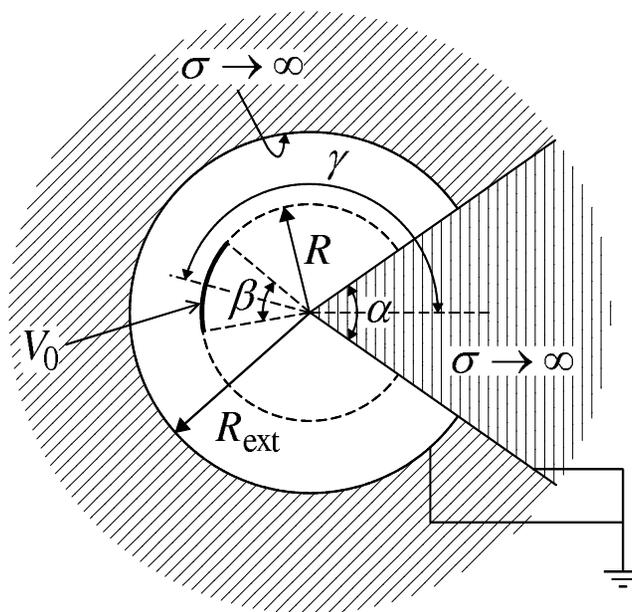
Figure 7.9: Capacitance associated with an edge.
