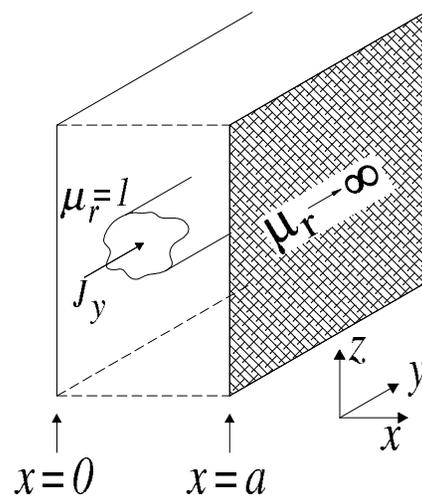
Figure 6.2: Magneto-quasi-static example for the use of Green’s function.
