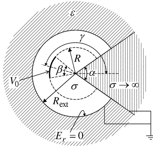
Figure 7.12: Resistor with an “edgy” electrode.
