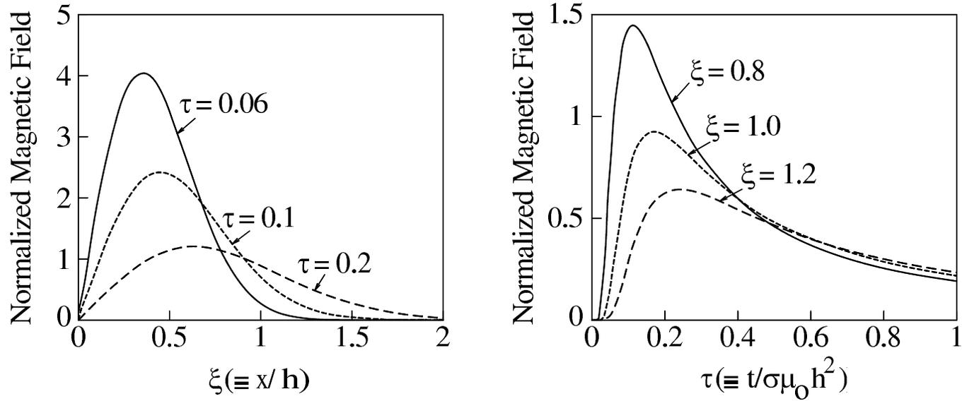
Figure 4.5: Normalized magnetic field at various times (left) and locations (right).
