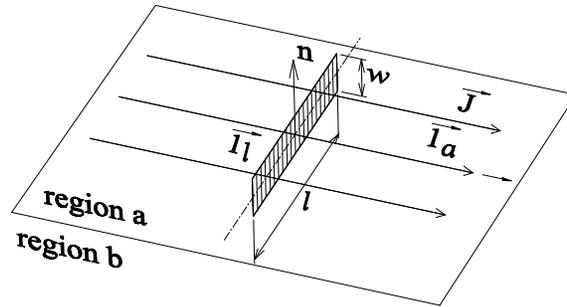
Figure 1.7: Discontinuity of the tangential magnetic field is linked with a surface current density.
