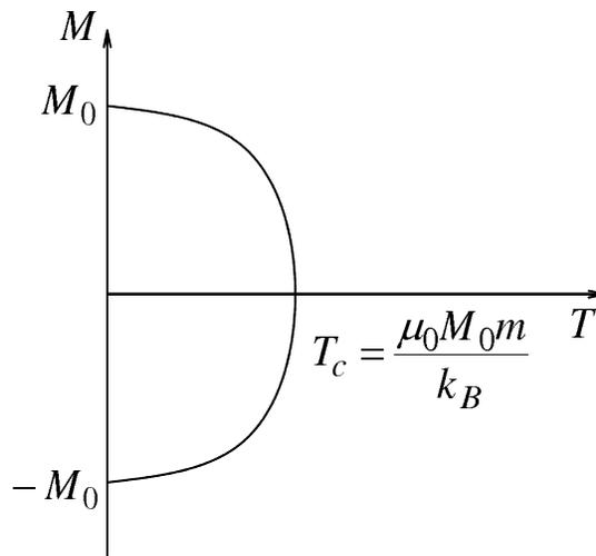
Figure 7.A.3: Magnetization field as a function of temperature.
