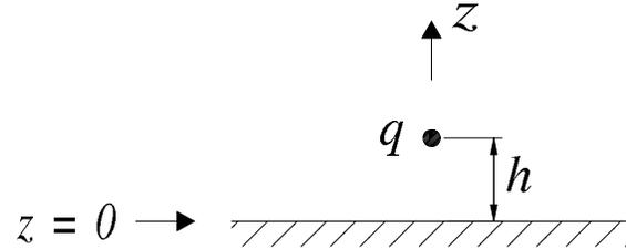
Figure 6.4: Point-charge,  $q$ , at a height  $h$  above a grounded surface.
