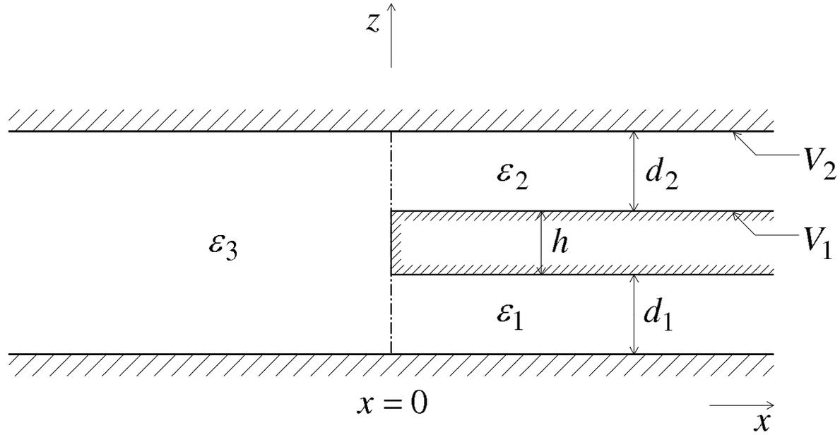
Figure 5.6: A three electrode system: the lower one is grounded on the central one at voltage  $V_1$  is imposed and  $V_2$  on the topelectrode. Note that in each region the dielectric coefficient is different.
