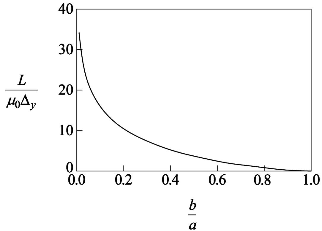
Figure 6.3: Inductance  $L$  as a function of the width of the strip ( $b/a$ ).
