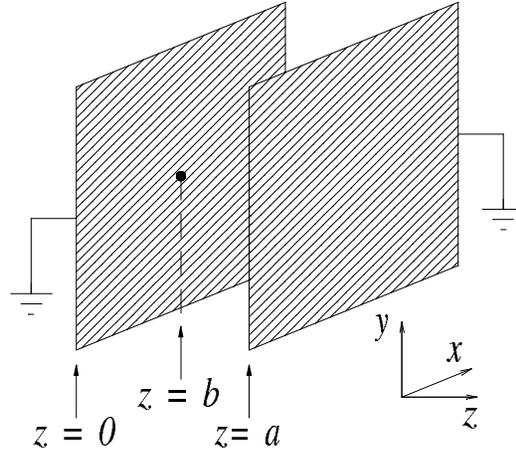
Figure 6.5: A point charge located between two parallel metallic plates.
