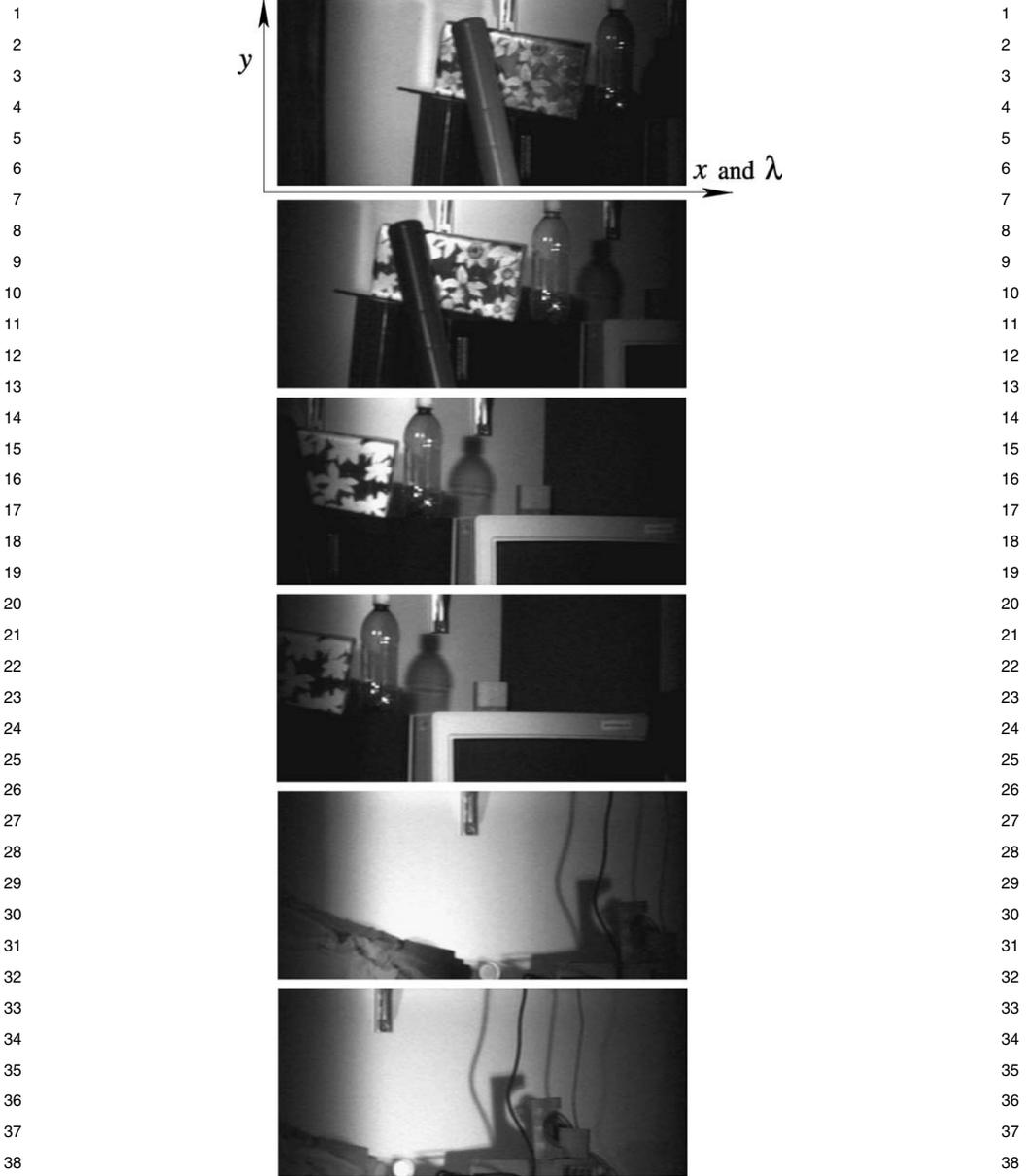
**Figure 8.17** Frames 29, 32, 38, 40, 60, and 64 of a sequence [32] taken through the linear variable interference filter. The left of the FOV senses the energy density at 700 nm, while the right senses it at 400 nm. The spatial features of the scene are clearly seen.
