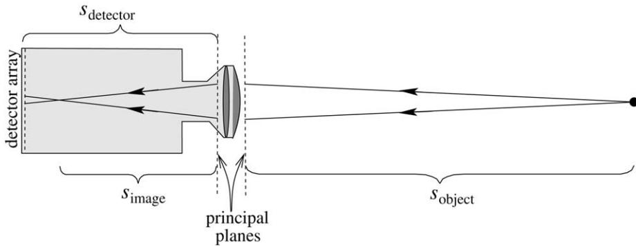
**Figure 8.3** Geometry of a simple camera system.
