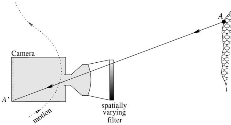
**Figure 8.2** Scene point  $A$  is imaged on the detector at  $A'$  through a spatially varying filter attached to the camera. As the imaging system moves [31], each scene point is sensed through different portions of the filter, thus multiple measurements are obtained under different optical settings.
