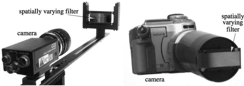
**Figure 8.13** Two generalised mosaicing systems [31–33]. (Left) A system composed of a Sony black/white video camera and an extended arm which holds the filter. (Right) A system that includes a Canon Optura digital video camera and a cylindrical attachment that holds the filter. In both cases, the camera moves with the attached filter as a rigid system.
