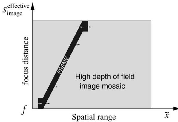
**Figure 8.5** Each frame has a spatially varying focus. Generalised mosaicing of such frames extends both the FOV and the DOF.
