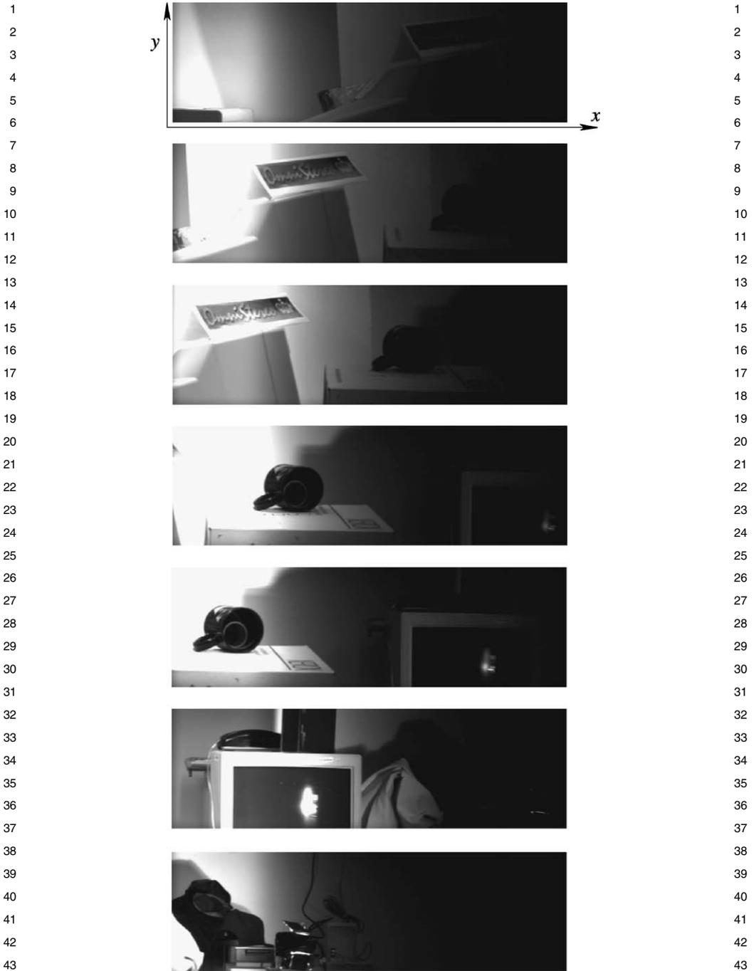
**Figure 8.15** Frames 4, 9, 11, 15, 17, 23, and 31 from a sequence taken with a linear variable density filter [33]. Scene features become brighter as they move leftwards in the frame. Bright scene points gradually reach saturation. Dim scene points, which are not visible in the right-hand side of the frames, become visible when they appear on the left.
