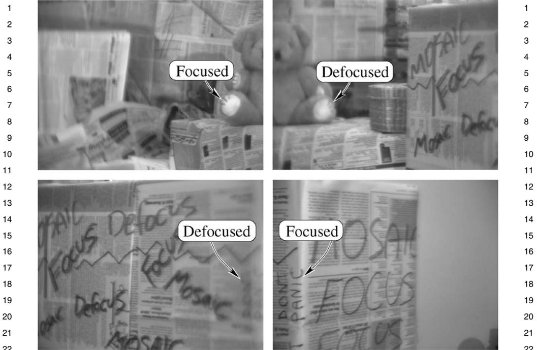
**Figure 8.10** The frame in which an object is focused depends on its position in the frame. The teddy bear is focused only when it appears on the right-hand side of the frame's FOV. The words 'don't panic' are focused only when they appear in the left-hand side of the frame's FOV.
