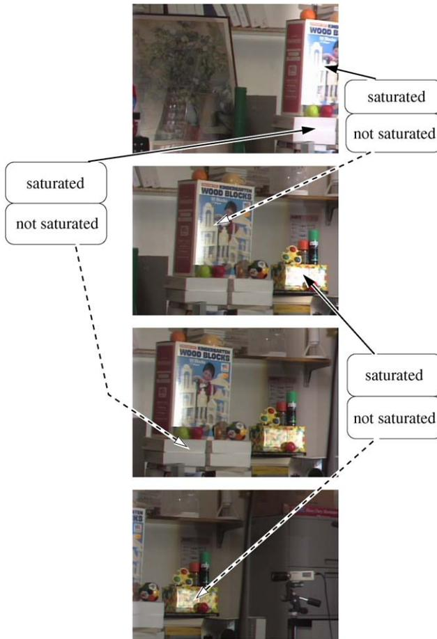
**Figure 8.19** A few frames from a sequence [34] taken through a mounted filter. The filter has spatially varying attenuation and polarisation characteristics. The effective filtering variations are gradual and not easily visible, due to defocus blur of the filter. Nevertheless, the spatial variations make objects appear brighter on the right-hand side. Thus saturated pixels on the right appear unsaturated in other frames, in corresponding left-hand side pixels.
