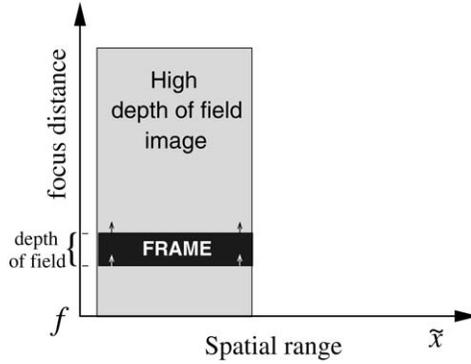
**Figure 8.4** An image frame has a limited FOV of the scene (marked by  $\tilde{x}$ ) and a limited DOF. By fusing differently focused images, the DOF can be extended by image post processing, but the FOV remains limited.
