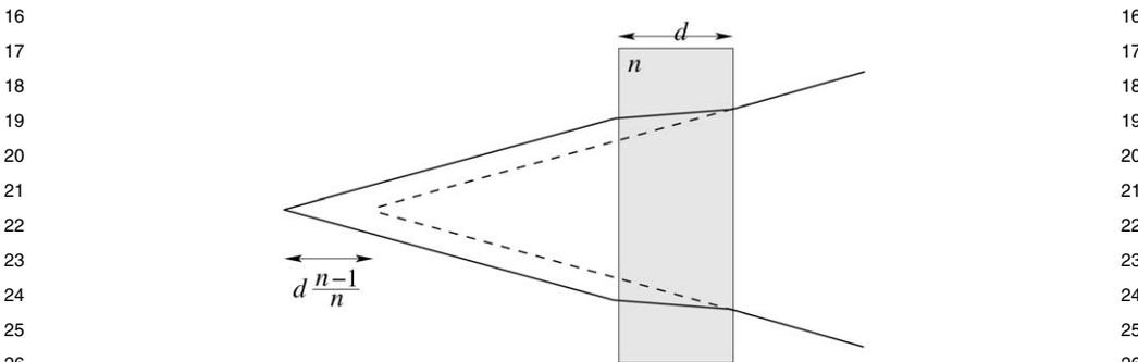
**Figure 8.7** A dielectric with refraction index  $n$  and thickness  $d$ . If it is placed before the detector, it shifts the focused image point away from the imaging optics.
