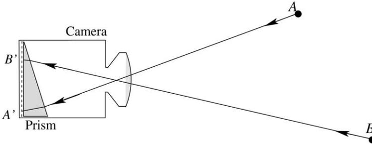
**Figure 8.9** The focus settings can change across the frame’s FOV by placing a transparent object with variable thickness on the detector. Here, a wedge-prism is placed on the detector array, such that both objects A and B are focused even-though they are at different distances from the camera.
