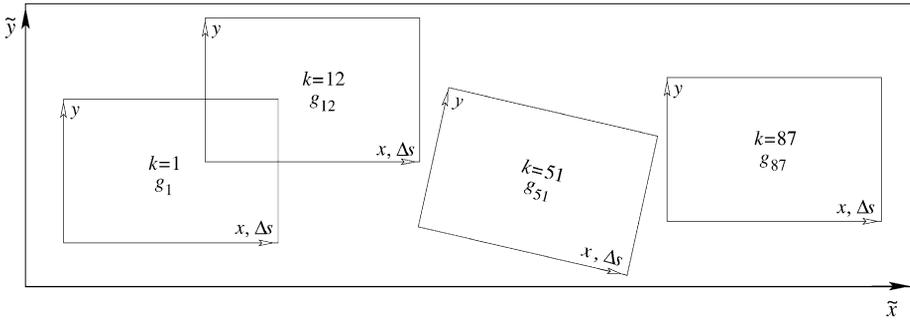
**Figure 8.8** The coordinates  $(\tilde{x}, \tilde{y})$  denote the position of a scene point in the global coordinate system of the mosaic [32]. The mosaic is composed of raw frames indexed by  $k$ . The intensity in a raw frame is  $g_k(x, y)$ , where  $(x, y)$  are the internal coordinates in the frame. The axial shift  $\Delta s$  of the SLC is a function of  $(x, y)$ .
