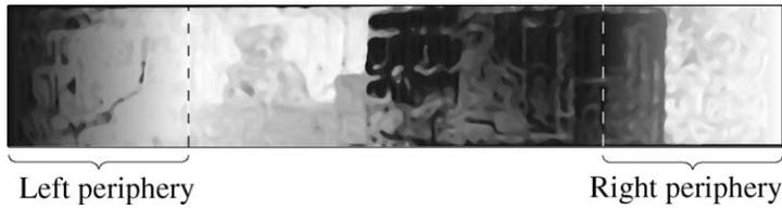
**Figure 8.11** A map equivalent to a rough object distance, estimated in an experiment. Brighter pixels correspond to objects at larger object distances.
