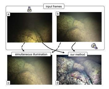
Fig. 5. Result of an underwater experiment using multidirectional illumination. (a) and (b) Raw frames. (c) Image as if the scene was illuminated by both sources simultaneously, generated by combining frames (a) and (b). (d) Result of our method.
