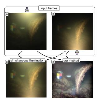
Fig. 4. Result of an underwater experiment using multidirectional illumination. (a) and (b) Raw frames. (c) Image as if the scene was illuminated by both sources simultaneously, generated by combining frames (a) and (b). (d) Result of our method.
