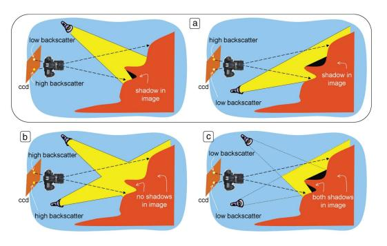
Fig. 3. (a) Underwater scene illuminated from two different directions. The shadows vary, as well as the intensity of the backscatter in each pixel. (b) Same scene, illuminated with both sources simultaneously. There are no deep shadows, and there is high backscatter. (c) Desired outcome of image fusion. Both shadows appear, while the backscatter component is lower.
