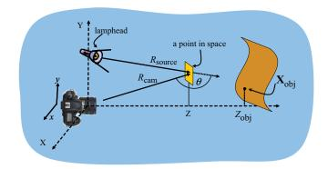
Fig. 1. Underwater camera imaging setup with an artificial light source [16]. The variables are detailed in the text.
