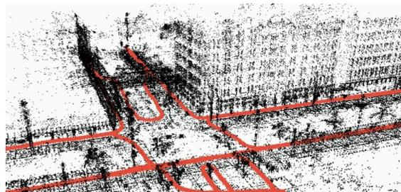
Figure 1. Given a series of 2D images and taken by a camera from different positions, the iterative Bundle Adjustment (BA) process evaluates the 3D locations of the objects in the images (in black) and the camera’s poses, as seen in the red trajectory. We propose a method to accelerate the process by reducing the number iterations required for the solving.
