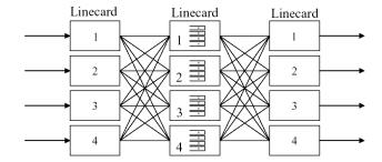
Fig. 1. Load-balanced switch architecture
