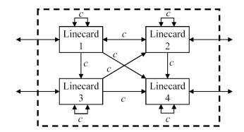
Fig. 3. Example of load-balanced routing network
