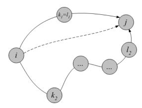
Fig. 4. Load-balancing example illustrating Proposition 12. The dashed line between i and j is a direct path. The two other paths are load-balanced paths in  $P_{LB}(i,j)$ . In the first load-balanced path  $k_1=l_1$ , in the second  $k_2 \neq l_2$ .
