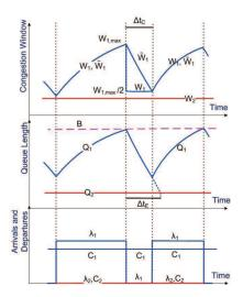
Fig. 3. Starvation mode for two TCP flows in a  $2 \times 1$  MWM switch
