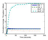
Fig. 4. Simulation of OQ and IQ-iSLIP cumulative average throughput.
