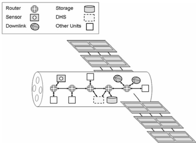
Figure 1: Elongated Shape of a Typical Satellite
