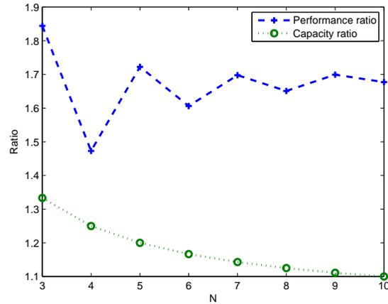
Fig. 7. Comparison of the performance ratio and the capacity ratio of the Torus and the Mesh using average online performance random-greedy algorithm.
