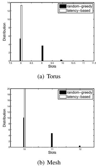
Fig. 6. Period length distribution with the *permutation* traffic pattern. In all cases the latency-based algorithm achieves a better distribution.
