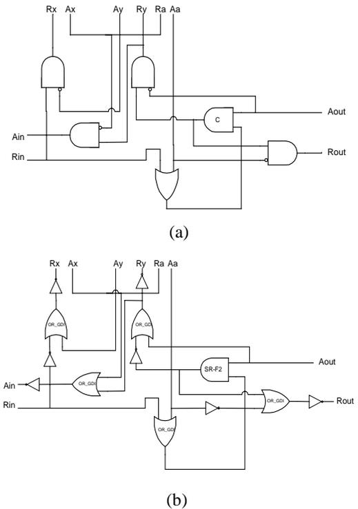
Fig. 12. Bundled-Data Filter Controller: (a) CMOS-based, (b) GDI-OR-based.
