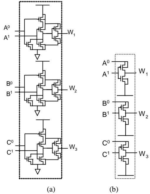
Fig. 19. ORN subnet Full Adder (a) CMOS based (b) GDI based
