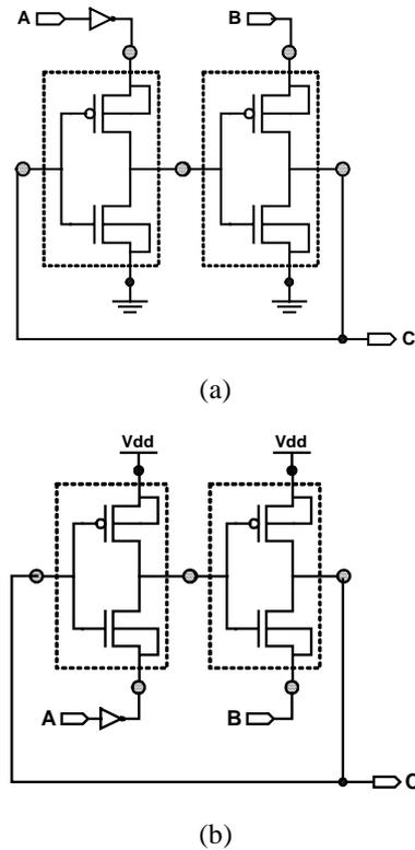
Fig. 6. GDI SR-Latch circuits using (a) F1, (b) F2 functions
