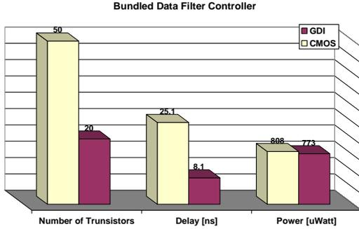
Fig. 13. Simulation results for Bundled-Data filter controller.
