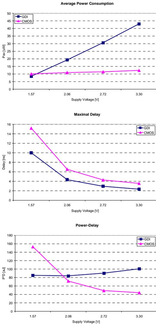
Fig. 10. Simulation results of operation at various supply voltages of 3-input C-element.
