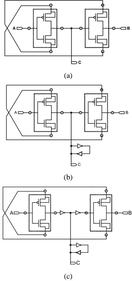
Fig. 3. GDI implementations of C-element: (a) dynamic, (b) static, (c) buffered static
