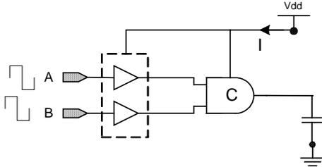
Fig. 8. Simulation environment of C-element.
