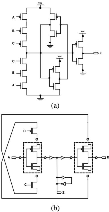
Fig. 4. Three-input C-elements in (a) CMOS and (b) GDI
