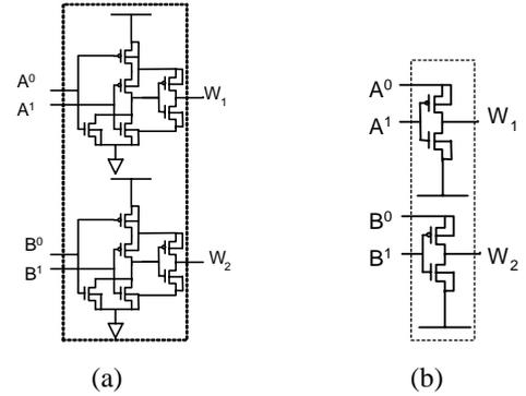
Fig. 15. ORN subnet (a) CMOS based (b) GDI based
