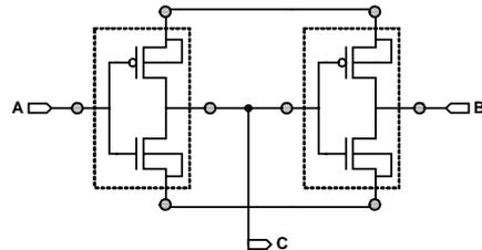
Fig. 7. GDI implementations of dynamic C-element with inverted input A.
