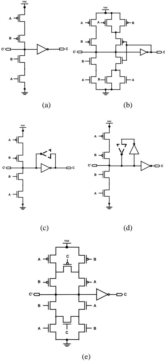
Fig. 2. CMOS C-element Circuits: (a) dynamic, (b) conventional, (c) weak feedback, (d) static, (e) symmetric.
